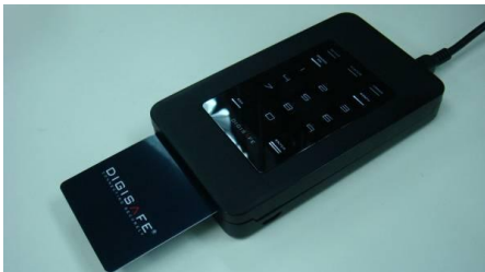
Insert the smart card into the smart card slot with the contacts facing down and the word "DigiSAFE" on the card facing up
